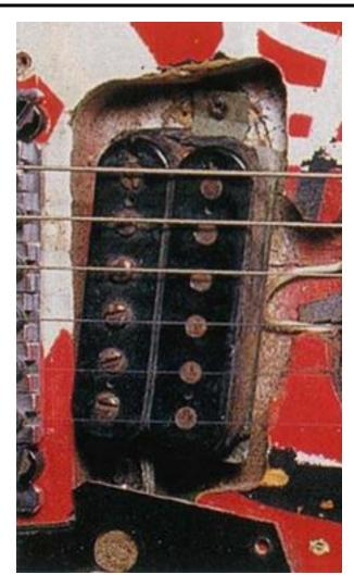
Use a single 500K pot for this pickup. See the wiring diagram to the right.
