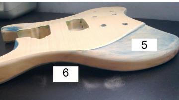
You can see blue remains on the body before painting. This is the remains of the first attempt to paint the body with a blue transparent lacquer. The problem is that the body is made of 7 different pieces: 3 for the base, 2 for the "arch top", 1 veneer and one very thick coat. They react different with the paint, at places were the wood was cut, and the result is awful. This is why I ended up with an opaque paint.
