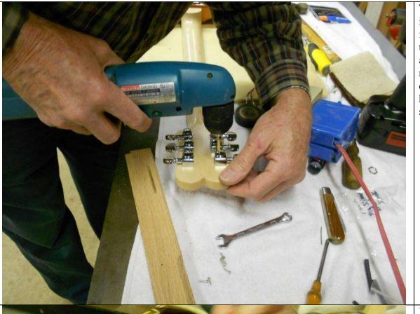
The only thing that is not stock in the first assembly are the tuners. These are Grover rotomatics. Here, dad is drilling pilot holes for the tuner screws.
