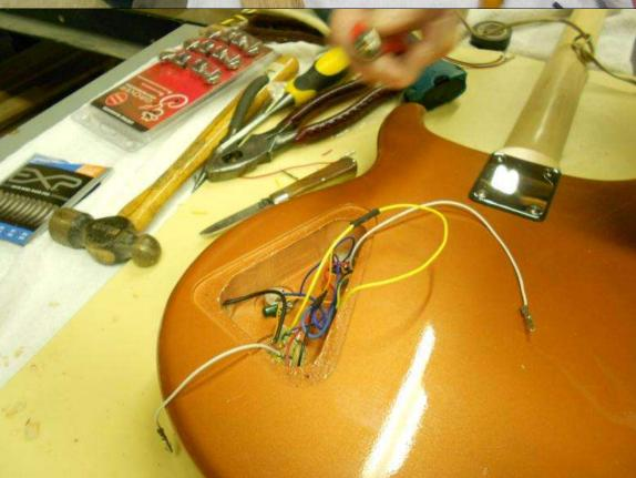
Here is the electronics work and shows our one "#\$#\$#\$Q\$#@ moment". When hammering in the cams for the Tailpiece, we let a wire hang loose and it scratched the back finish. See bottom middle of the photo. That's the price we pay for the quick paint job, but it gives the guitar character I guess.
