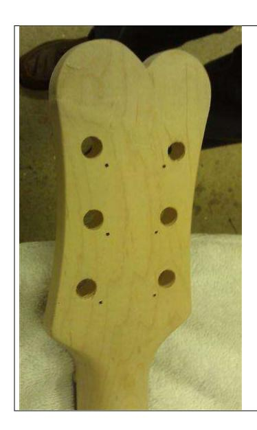
The new headstock is based on a large letter "B". I printed a template from the computer of a giant Arial Font bold B, and we rough cut with a jig saw and then various sanding levels to smoothness. So no it's not a rear end, or a symbol for breasts, it's a B. But hey this is rock and roll so whatever floats your boat !! ☺
